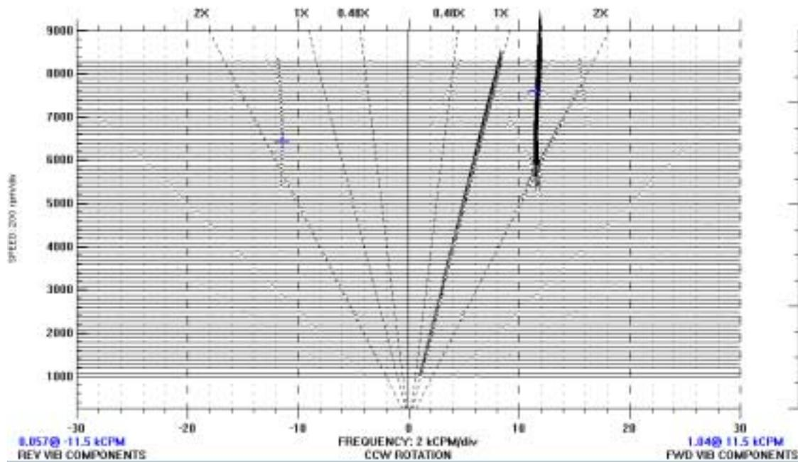
**Figure 3. Cascade plot showing changes in frequency spectrum as running speed increases.**
