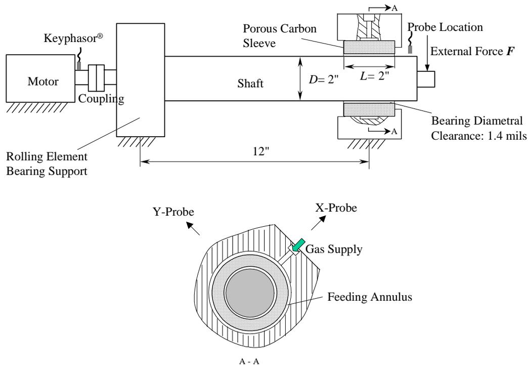
**Figure 1. Gas bearing test stand.**
