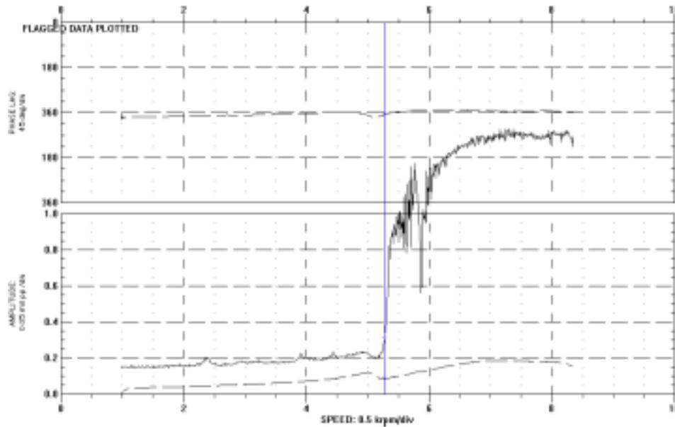
**Figure 2. Bode plot depicting typical air hammer onset.**
